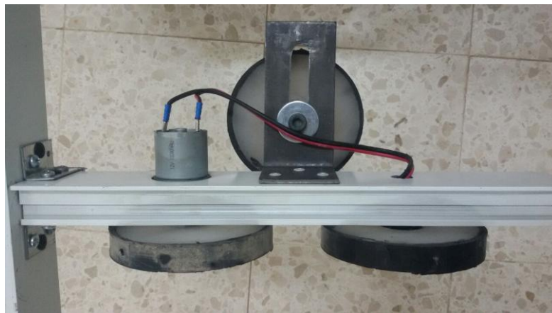
Figure 3-4: wheels and motor of structure
