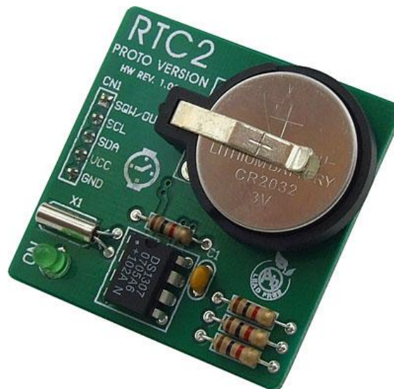
Figure 4-12: Real time clock circuit
